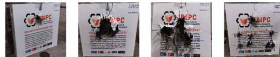
HUB 12.7 x 99 API M8 / 14.5 x 114 API M32. SHATTERING FIRE TO PIERCE ARMOR
