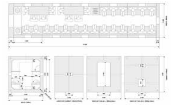
A sample of a possible arrangement. Five individually fitted segments with doors and escape entrance.
